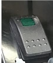
Engage/disengage the drum rotation
